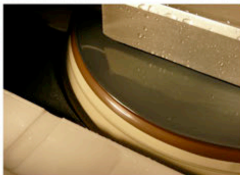
Fig 4 : Exakt band saw (above) and grinding system (below)
